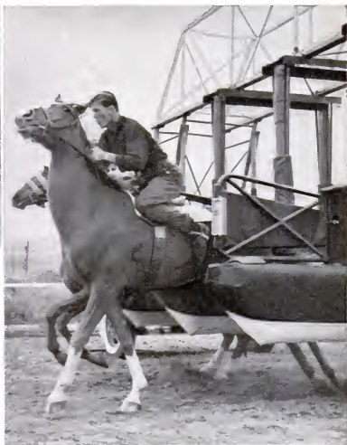
Testing the new race-track starting barrier that dispenses with the need of grooms to keep horses from backing up
